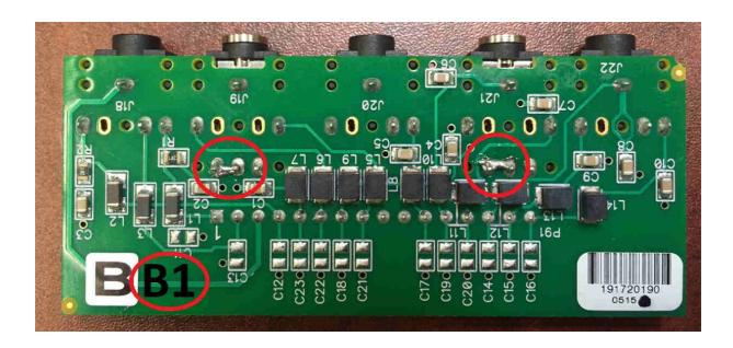
Test procedure: visually inspect the solder jumper at both locations, checking carefully to ensure nothing besides the two pins are shorted together.
